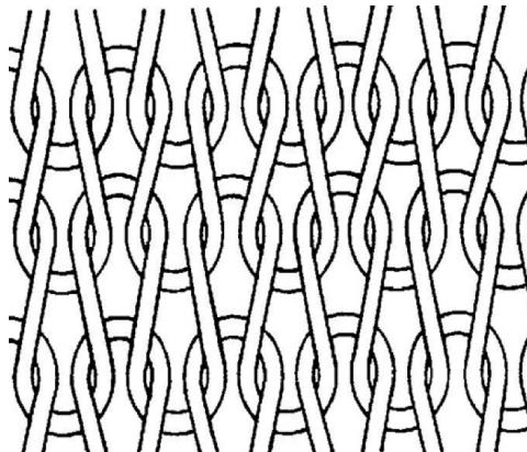
**Specifications:** Knit from 21/1's core-spun yarn, a core of 99 denier crystalline silica fiber within a sheath of modacrylic fiber. Fabric weight is 5.5 ounces per square yard (+/- 0.5 oz.). Blend level is 61% modacrylic / 39% crystalline silica fiber.
